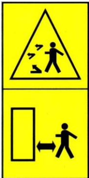
Fig. 2: Injury risk due flying fragments, chippings, ejected objects, etc. Other persons and animals – keep the safety distance to the machine.
