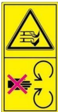
Fig. 4: It is not allowed to put hands or legs into the working space of the mowing knife – danger of cutting.
